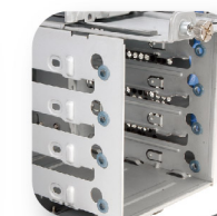
Optional 4-bays 3.5" HDD cages with anti-vibration absorbers
